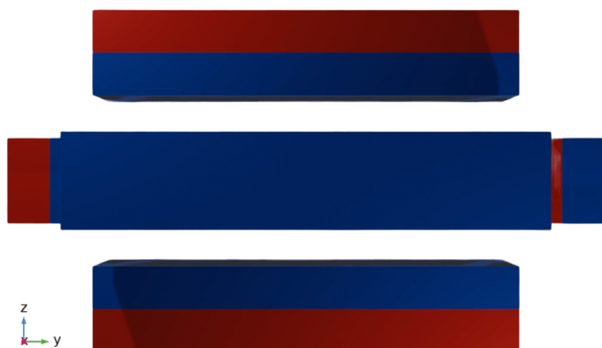
Figure 20: Illustration of the third presented model, where on each side of the quadrupole a 'closing' magnet is introduced. The N-poles are coloured red and the S-poles are coloured blue. Illustration made in Blender software.
