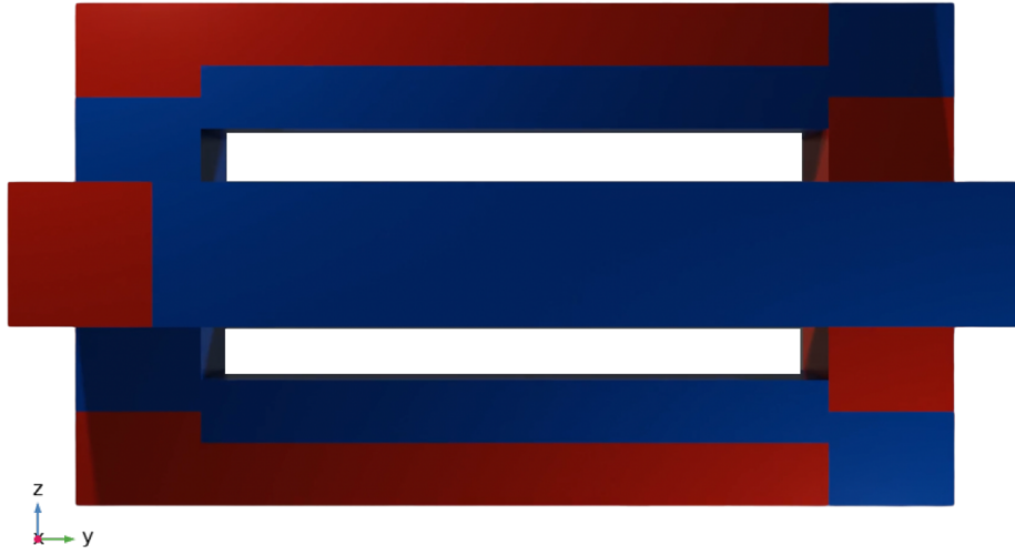
Figure 14: Illustration of the second presented model, where the shape of the quadrupole magnets is alternated. The N-poles are colored red and the S-poles are coloured blue. Illustration made in Blender software.
