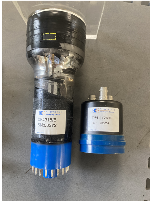
Figure 4: The type of photomultiplier tube and voltage divider attached to the BaF 2 crystals in the detectors
