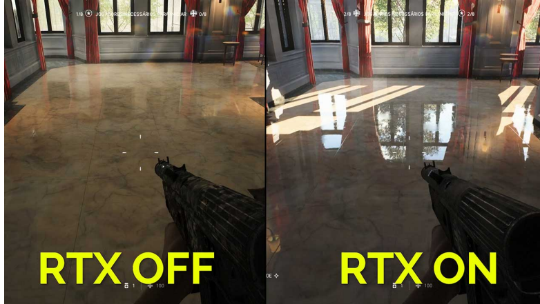
Figure 1: The difference between a scene without ray tracing and with ray tracing using Nvidia RTX [1].
