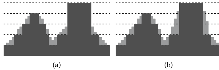
Figure 9.1: Different approaches to layer blending, (a) Current blending method which only blends between consecutive layers, (b) Blending method that blends between any two components.
