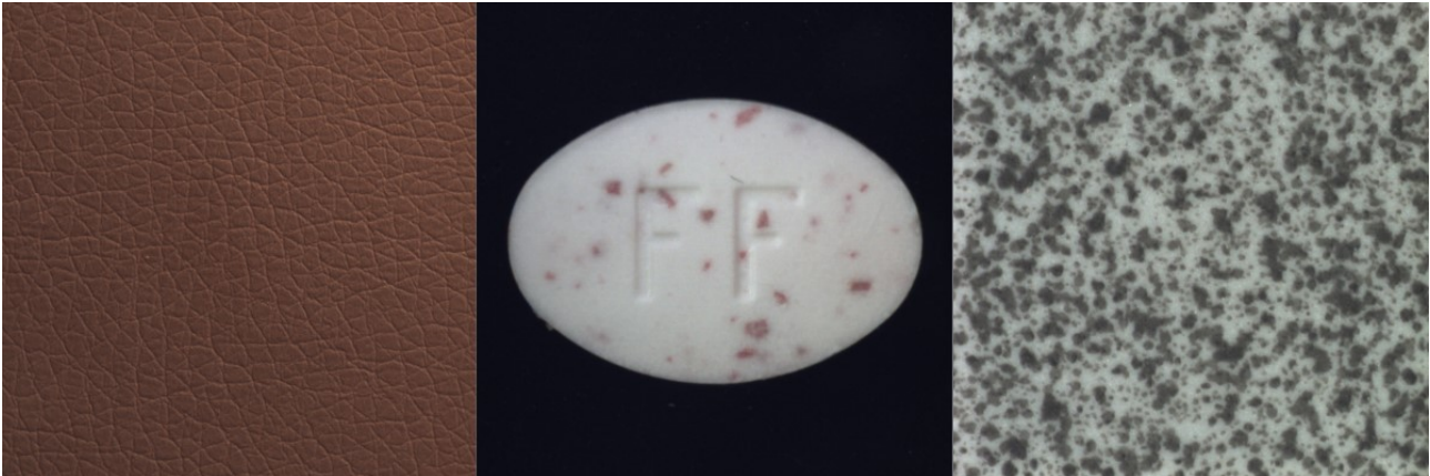
Figure 17: Some images of the MVTEC dataset showing non-defect samples. A sample of the "Leather" category is shown left, "Pill" in the middle and "Tile" on the right. Even though the objects are normal, they have random aspects that are hard to predict. This causes the IEM to assign them high energies, even though they do not have any defects.
