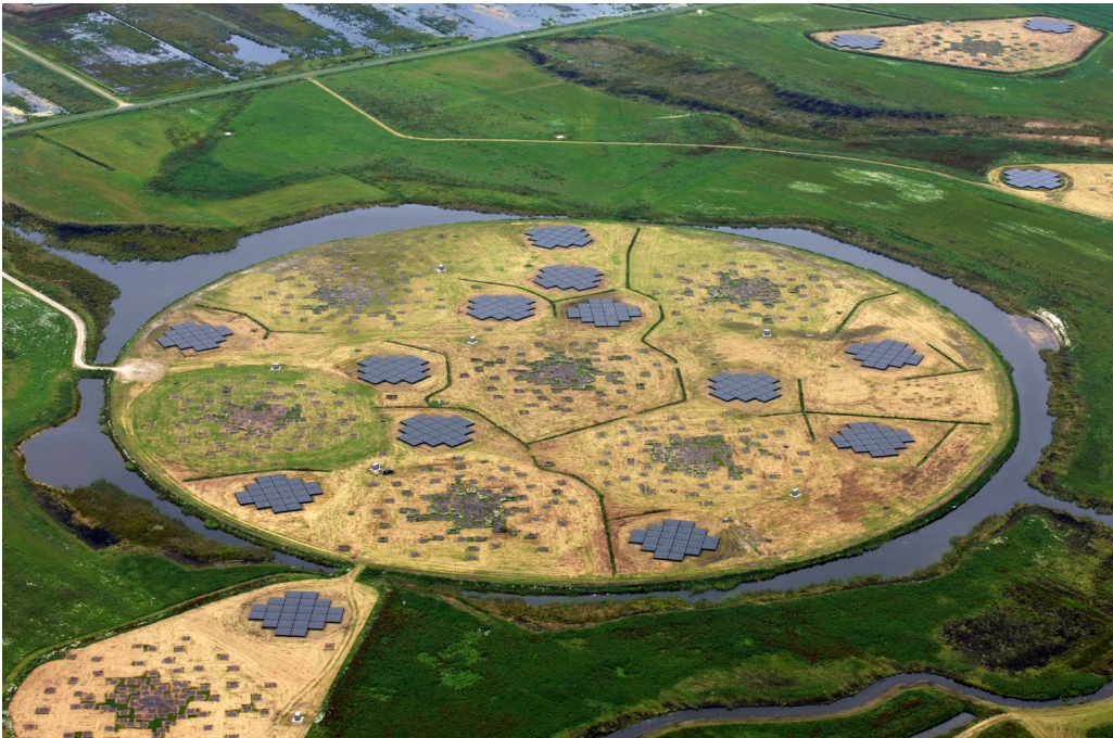
Figure 1.1.1: The LOFAR Superterp. The central six LOFAR stations visible with a few of the other stations in the LOFAR core visible in the foreground and background. Visible are high band antennas (HBA) in the form of hexagonal tile arrays and low band antennas (LBA) in the form of the 'haphazardly' arranged rectangles between each pair of hexagonal arrays. [11]
