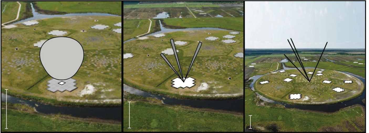
Figure 9: Illustration of different beam responses that include elements of the HBA antenna in the LOFAR core. Relevant HBA elements are highlighted in white, while the corresponding beam can be seen in grey. The left image shows the beam of a single tile in the HBA array, the middle image shows three beams from the combination of all 24 HBA station tiles and the right image shows four simultaneous beams formed by combining HBA tiles from all 24 core stations (not all are displayed; Stappers, B. W. et al. 2011 ).
