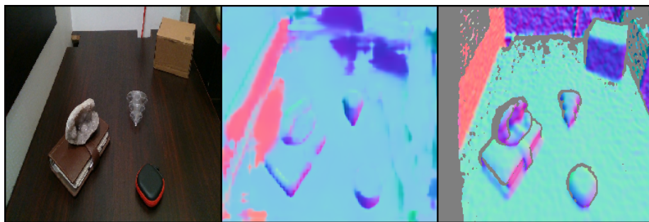
(a) Left: Input image, Center: Normals predicted by ResNet-50 + PSA model, Right: groundtruth.
