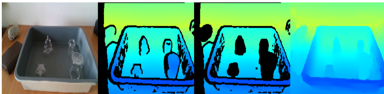
(a) First: Input RGB image, Second: groundtruth, Third: Input depth image, Fourth: depth estimated with ResNet-50 + PSA model.
