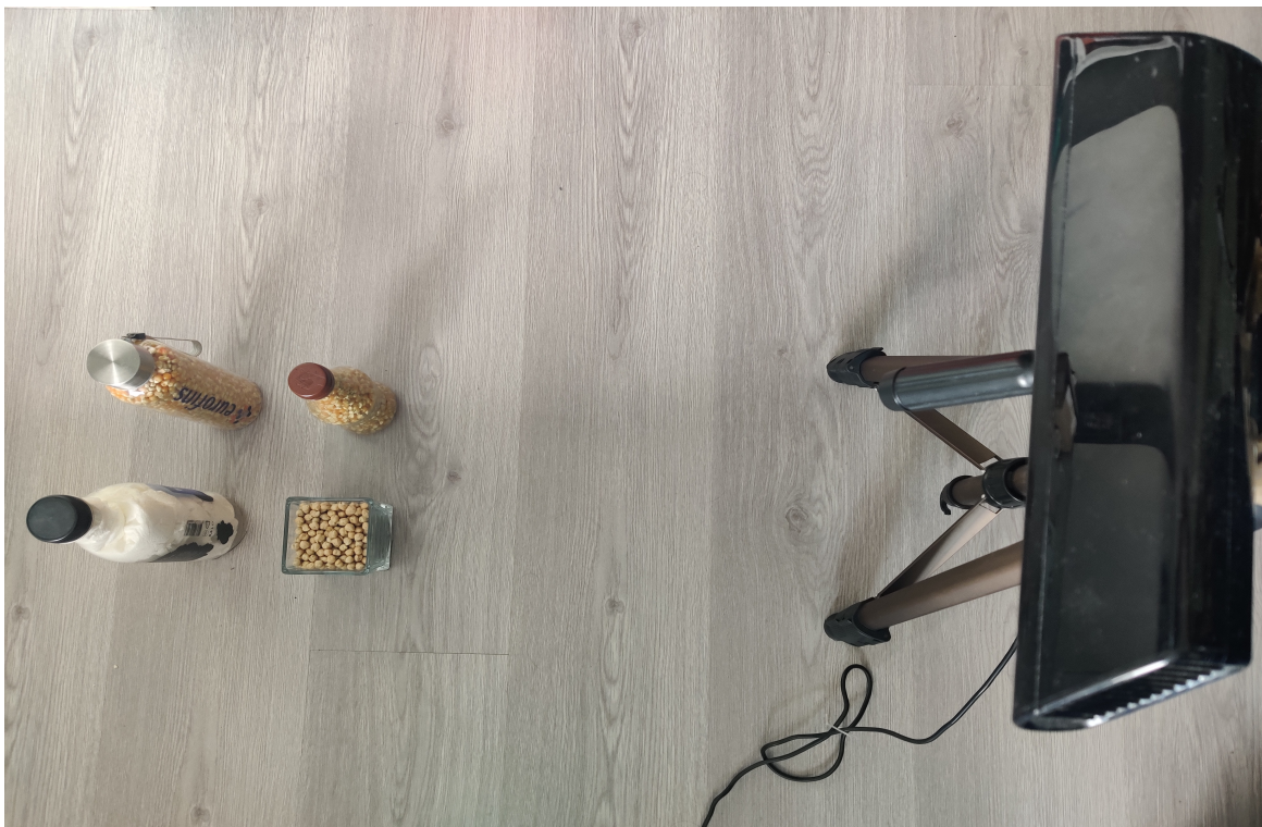
Figure 11: Top view image of the transparent objects filled with various things along with the tripod and the Kinect-v1 camera.
