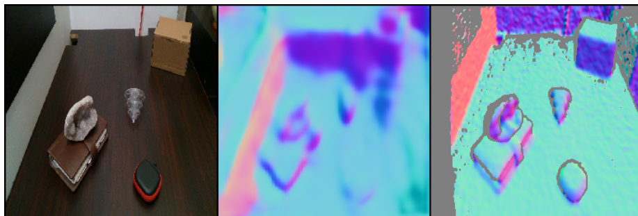
(b) Left: Input image, Center: Normals predicted by DRN model, Right: groundtruth.
