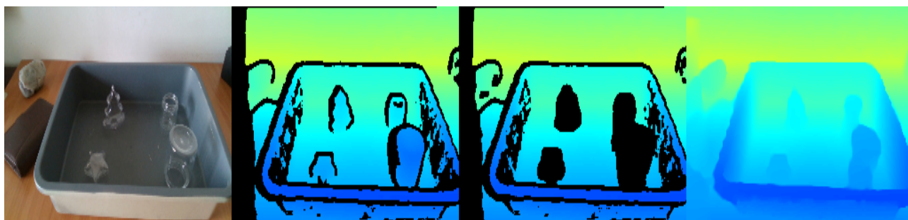
(b) First: Input RGB image, Second: groundtruth, Third: Input depth image, Fourth: depth estimated with DRN model.
