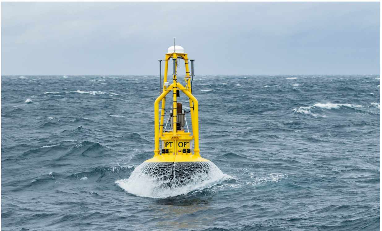
Figure 1.1: An operational point-absorber wave-energy-converter deployed by Enel Green Power in Chile, 2021 [WEC, 2021].
