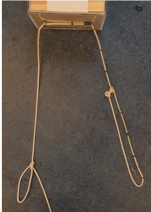
Figure 4.3: The cable configuration, with a bowline knot on the left (for its strength), connected through both connectors to the tarbuck knot on the right, with the regular interval markings visible. (Note that the right connector is substituted with tape in this image, but normally it is identical to the left connector).
