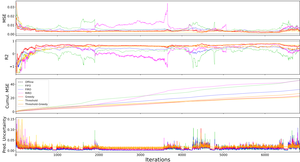
Figure 5.1: Comparison of models after basic hyperparameter tuning. The x-axis denotes the iterations over the training set, and the y-axis the performance of respective metrics on the testing set in each moment. The baseline models are denoted by dotted lines and uncertainty models by full lines. The graphs of MSE, R^2 , and predicted uncertainty were truncated to make the graphs more interpretable.
