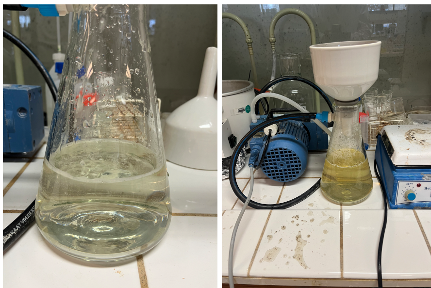
Figure 25: Resulting water in Büchner set-up after washing for one hour (left) and after one hour in the ultrasonic bath (right)
