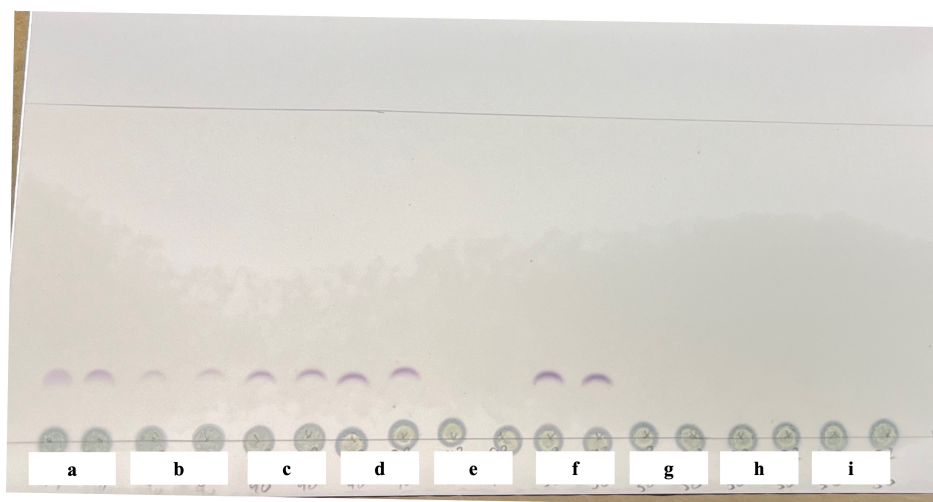
Figure 8: TLC organic acids assay showing the removal of acetic acid by vacuum distillation at differing temperatures over several cycles with 5 M (a) and 0.2 M (b) acetic acid, result after vacuum distillation at 40°C after the first (c), second (d), and third (e) cycle, and at 50°C after the first (f), second, (g), third (h) and fourth (i) cycle
