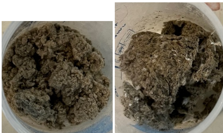
Figure 26: Picture of tertiary cellulose before (left) and after (right) washing
