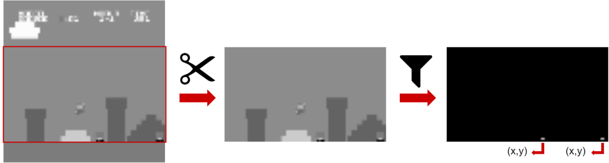
Figure 3.4: Processing pipeline for goomba detection. In short, first cut the frame, then mask for certain pixel values, and lastly, extract coordinates.
