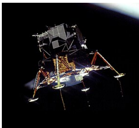
Figure 18: Apollo 11 Lunar Module Eagle in landing configuration[12]
