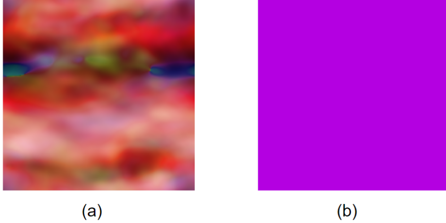
Figure 8: Visualizing the cubic magnetic sample at t = 1 \text{ ns} for (a) A_{\text{ex}} = 10^{-12} \text{ J/m} , and (b) A_{\text{ex}} = 10^{-10} \text{ J/m} . Where, colors represent different moment directions as seen through Figure 15.
