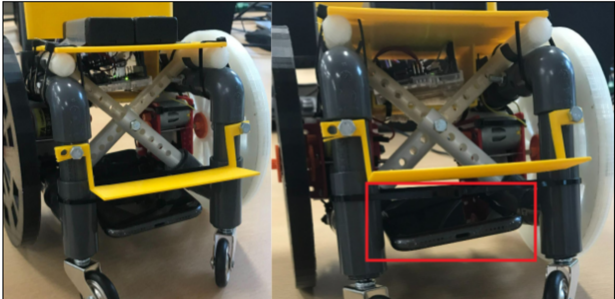
Figure 23: Heavy bottom structure.
