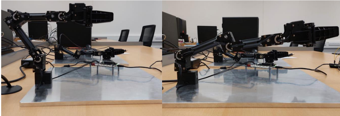
Figure 7 and 8. The gripper in its base (left) and giving (right) positions.
