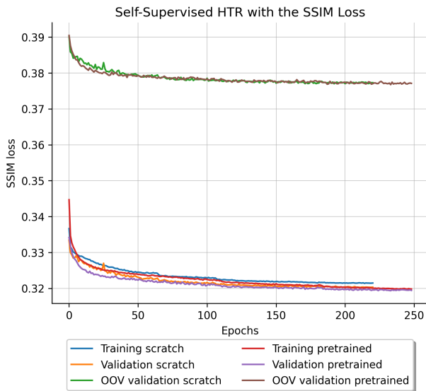
Figure 38: Self-supervised HTR trained with the SSIM loss on real IAM-HTR data loss curve
