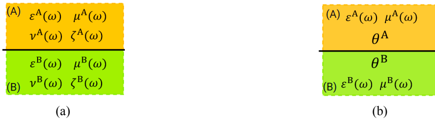
Figure H.1: (A) Interface conditions between two media characterized by surface conductivities, denoted as \sigma_s^A and \sigma_s^B respectively. (B) Interface conditions between two media are characterized by surface conductivities indicated by the different \theta values only.
