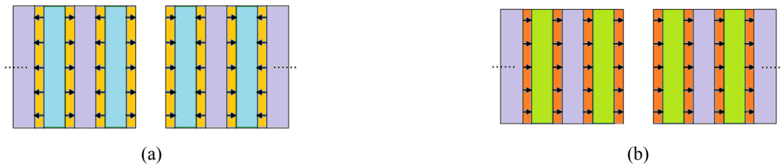
Figure 1.5: (A) Antiparallel configuration: magnetizations in the magnetic coatings on the TI layers are opposite. (B) Parallel configuration: magnetizations in the magnetic coatings on the TI layers are aligned.
