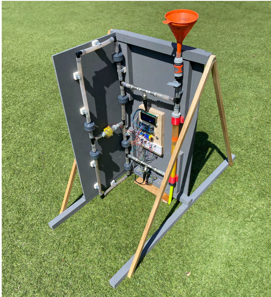
Figure 27: The final design of the small-scale PTO mounted onto a wooden frame.
