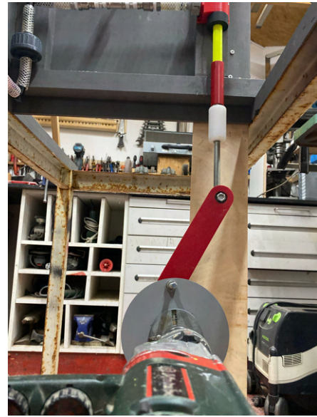
Figure 29: Front view of the linear reciprocating mechanism.
