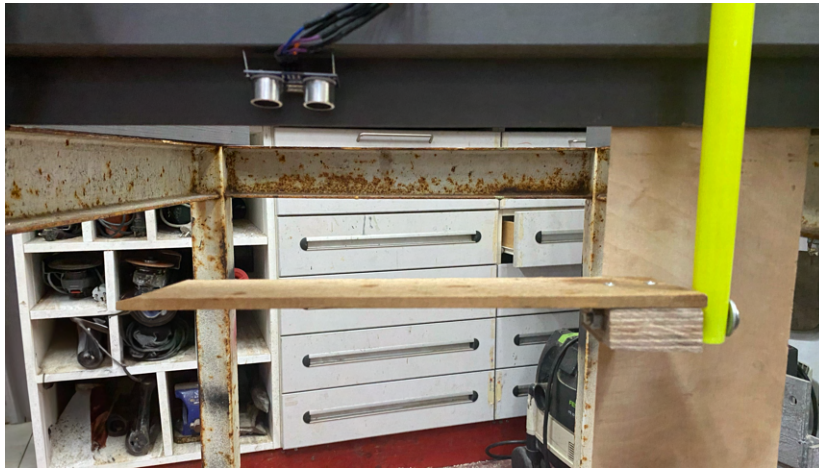
Figure 30: The ultrasonic sensor that measures the distance between the lower end of the piston and the construction frame.
