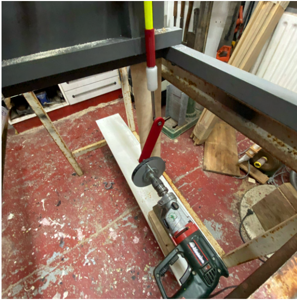
Figure 28: Isometric view of the linear reciprocating mechanism.
