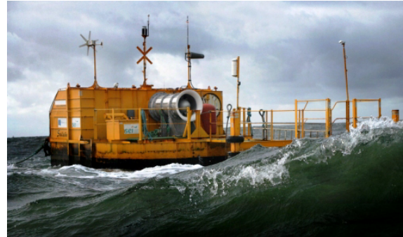
Figure 3: Example of an air powered PTO in a WEC.
