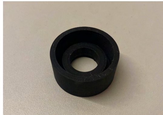
Figure 21: 3D printed adapter that is used to keep the O-ring in place.
