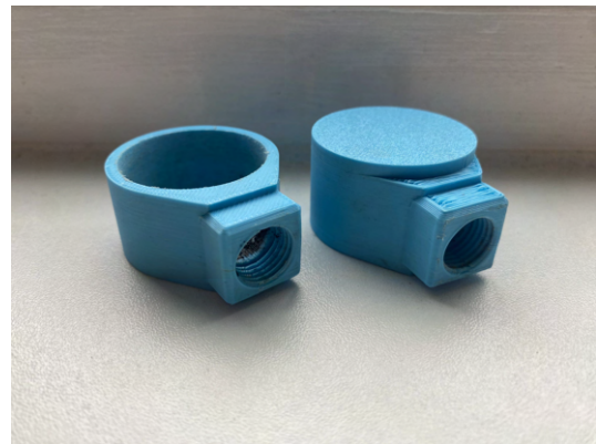
Figure 19: Two versions of the 3D printed adapter: one with cap and one without.
