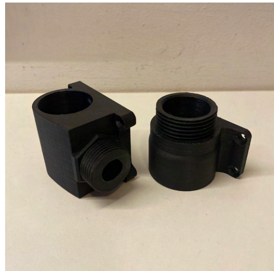
Figure 24: Updated 3D printed adapters with an integrated mounting plate.
