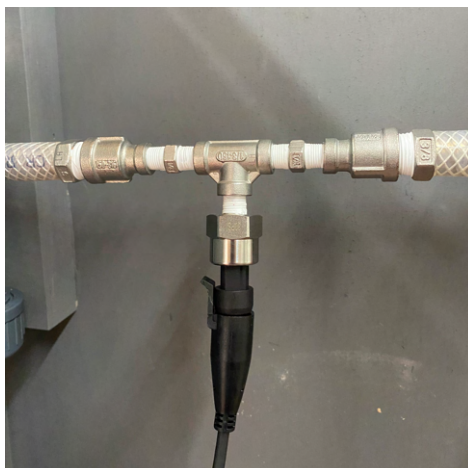
Figure 37: Several adapters were used to connect the P265 pressure transducer to the circuit.
