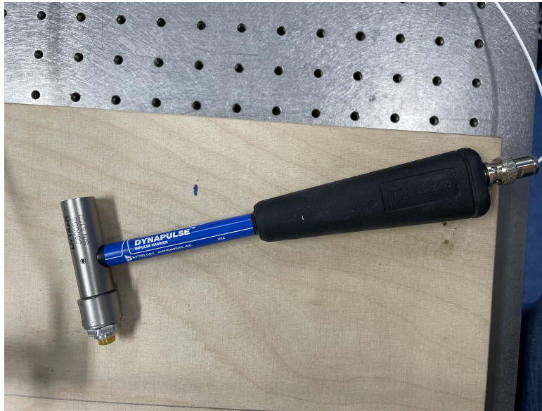
Figure 5: Hammer used for impact-testing.
