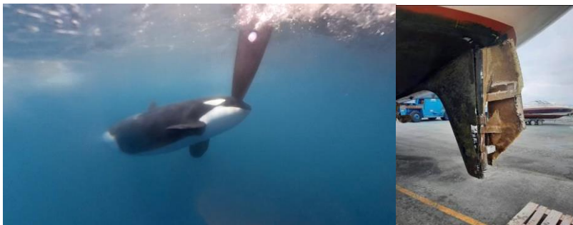
Fig. 2 Orca ramming the rudder of a sailboat and the damage it can lead to (Grimmett, 2021; Rusch, 2023)
