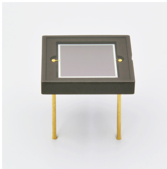
Figure 1: Hamamatsu S13360-6050CS used in the experiment [2]
