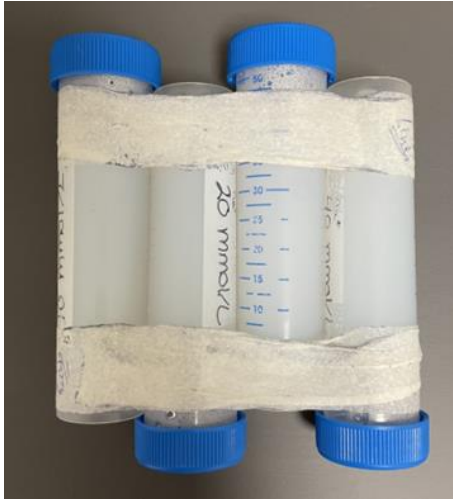
Figure 4: Reference phantoms of 10, 20, 30 and 40 mmol/L sodium in agar gel, respectively.
