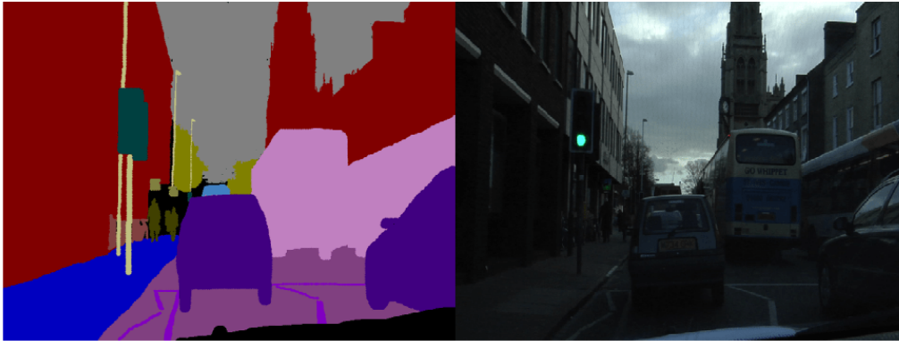
Figure 1.1: An example of a segmentation map, showing how a traffic image can be segmented into distinct objects. [18]
