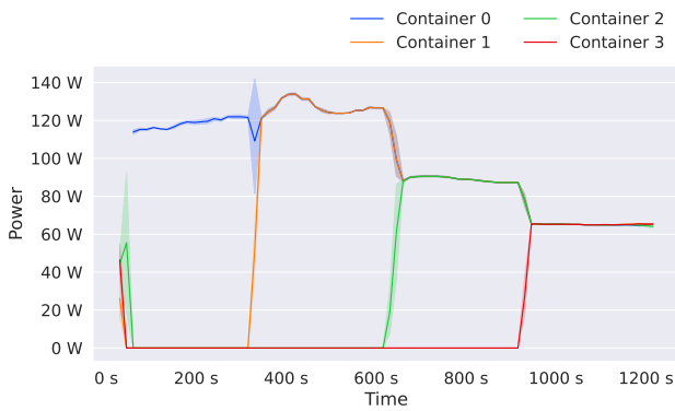
Figure 7.8: Power usage over time of the three repeated multiple-stressors tests.
