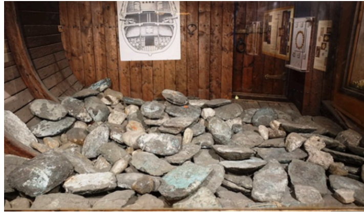
Fig 3 - solid ballast on medieval ship (Asiansealand, 2021)
