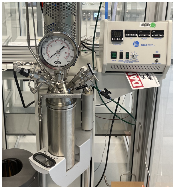
Figure 7: Parr 2 L batch reactor.
