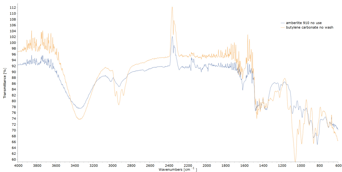
Figure 17: FT-IR Spectra Comparison: Unwashed vs. Ion-Exchanged Catalysts.
