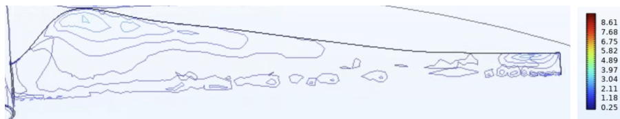
Figure 11: TKE plotted along one of the three blades. More intense turbulence is located on the trailing edge and the tip of the blade in the light blue shade and higher concentrated contour lines.
