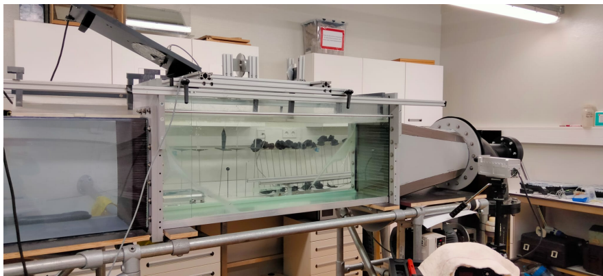
Figure 29: Photograph of the flow tank taken without a sample in it. The cross section is shown in the center of the photo.
