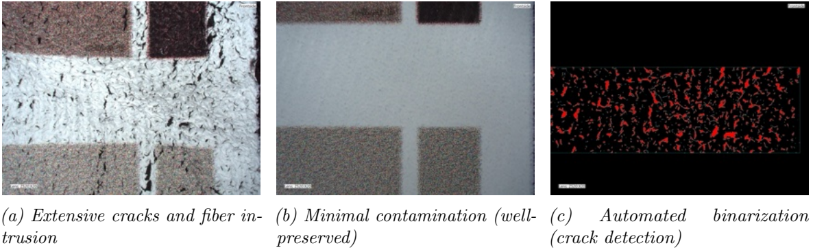
Figure 3.1: Microscopy of washed samples: (a) Cracking and fiber intrusion typical of Maegis A; (b) Well-adhered, undamaged print; (c) Automated detection of contaminant regions.
