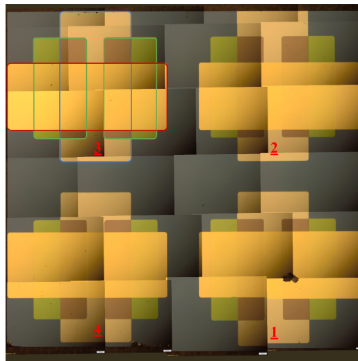
Figure 15: Image of working MTJ sample (8) obtained by stitching snapshots of optical microscope scans. The devices are labeled with numbers as they appear in characterization tests
