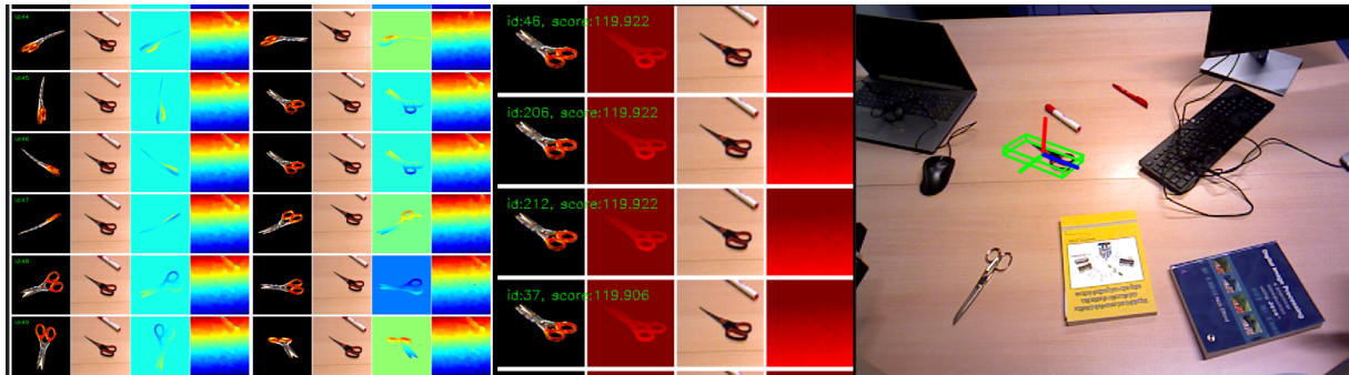
(a) Scissors object: sampled poses, depth refinement, scorer heatmap, final overlay.
