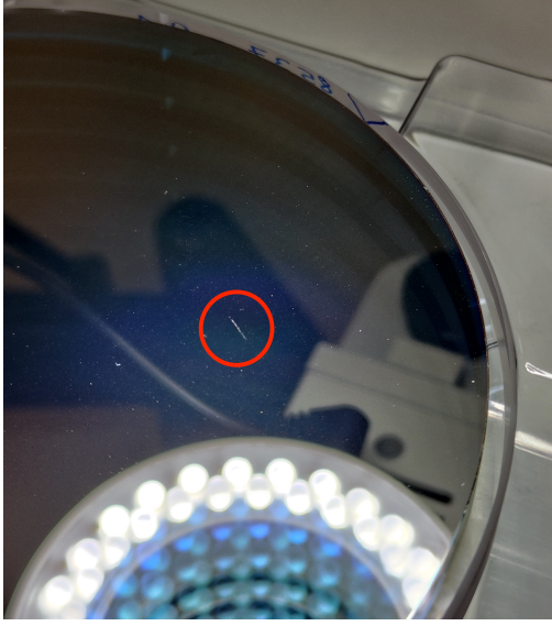
Figure 5.24: Defect in the shape of a line on face 2 of the I-long 8537-01 filter and marked by SCHOTT as number 5 in Figure 5.21.
