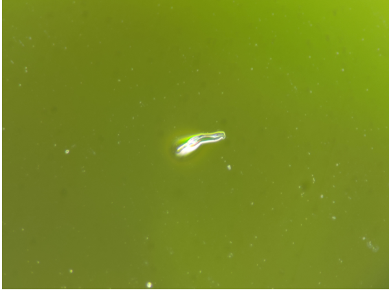
Figure 5.4: Defect with the size of 0.5 mm in length that creates a colorful pattern in the coating of the [FeII] filter with serial number SN31. Marked by Cilas as L0.016 in Figure 5.3.
