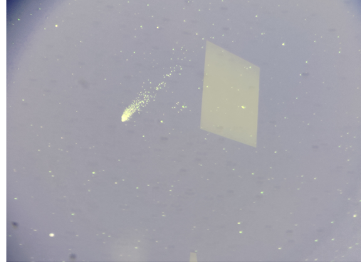
Figure 5.8: Region of clustered polishing dots on the [FeII] SN32 filter.
