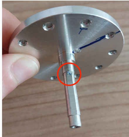
Figure 7.14: The component that got twisted because the thermal strap kept getting stuck, which required extra force to be applied on this piece whenever the motor rotated.
