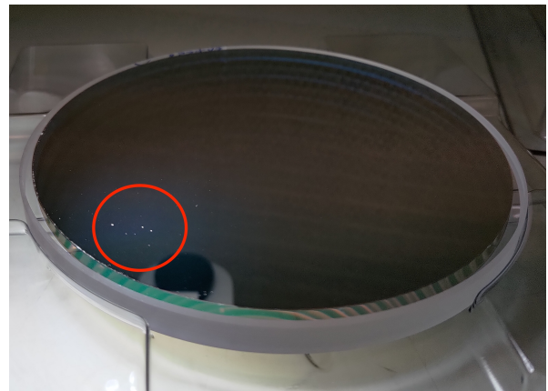
Figure 5.23: The defects marked by SCHOTT as numbers 5, 6, 7, 8, 9 in Figure 5.21, in the lower left part of the I-long 8537-13 filter on face 2.
