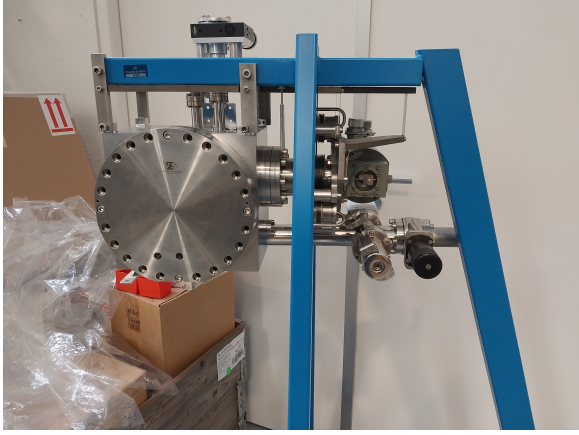
Figure 4.2: CRiSP viewed from the outside. The stepper motor is located on the top, while on the right, the mechanisms used to connect and control the vacuum pump and liquid helium source are visible.
