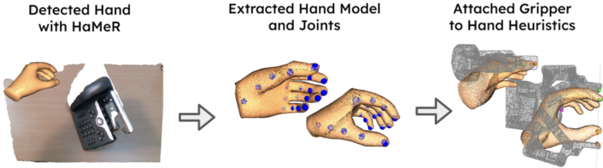
Figure 6: Converting human demonstrations into robot gripper trajectories. First, hand keypoints are extracted from video frames using the HaMeR model; then, a heuristic mapping is applied to convert the keypoints into gripper poses. [24]
