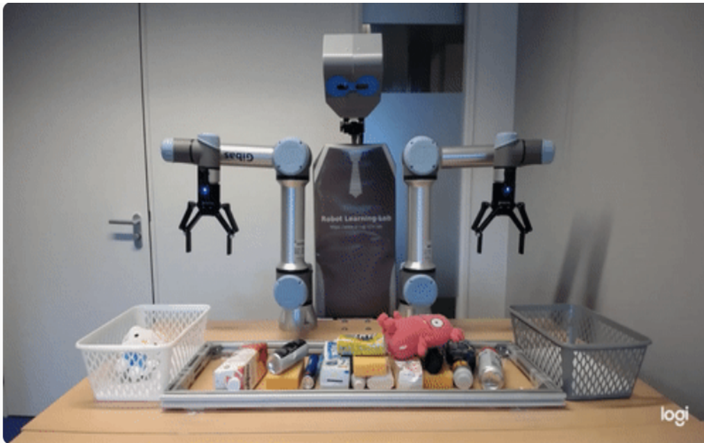
Figure 11: The dual-arm robot used in the robotics lab at the University of Groningen consists of two 6-DOF arms equipped with parallel-finger grippers. There is a RGB-D camera in the middle, placed above the workspace and angled downward to capture the interaction area.
