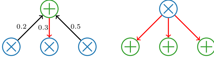
Figure 10: Left: sampling from the distribution encoded by a sum node — instead sample from the distribution encoded by one of its parents. Red edges point to the parent(s) chosen during the backwards sampling process. Right: sampling from the distribution encoded by a product node — sample from the distributions encoded by each of its parents.
