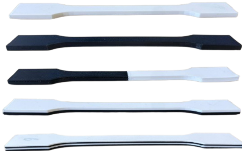
Figure 6: PLA, ABS, interlocking and layered dog bone structures, white representing PLA and black representing ABS material.
