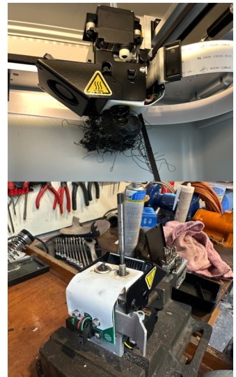
FIGURE 12 Both plastic and fiber clogs occurred regularly, resulting in printing delays.
