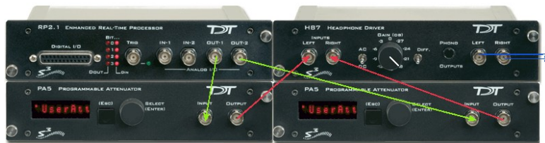
Figure 4.1 The Tucker Davis hardware and how it is connected.
