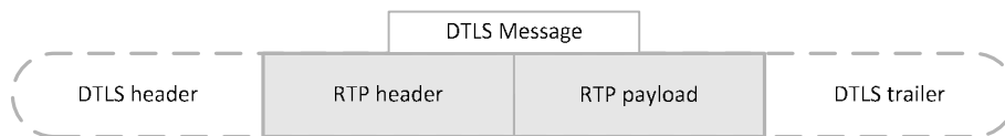
Figure 2.4 DTLS message structure: DTLS encrypts the whole RTP message and adds its own header and trailer
