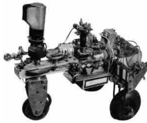
Figure 5: Grey Walter's 'tortoise', using behavior-based navigation.
