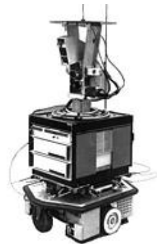
Figure 2: shakey, controlled by the symbolic program 'STRIPS'.
