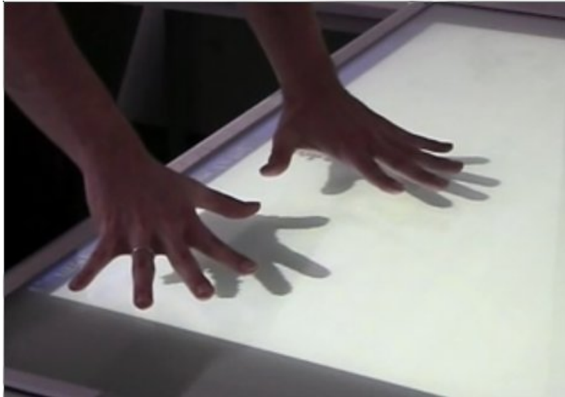
Figure 8.3: Shadow tracking. The shadows on the touch screen are actually rendered by the computer.
