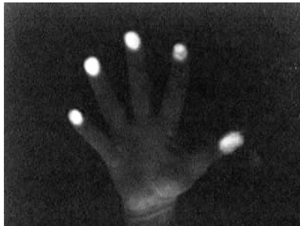
Figure 2.5: Frustrated reflection as captured by an infrared camera.
