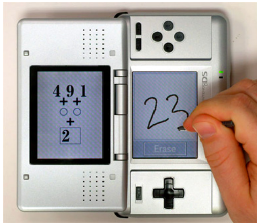
Figure 2.2: This gaming device has a resistive touch screen. ( Image from Nintendo )
