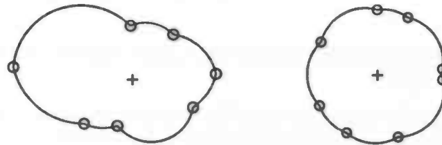
Figure 4.3: Two examples of the RBF-reconstruction from the vertices of a convex polygon. The function \phi(r) = r is used as the radial basis function. A single additional constraint (the + in the figures) is used.
