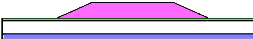
Figure 2: a transdermal drug delivery patch with a drug reservoir. From the top the different layers are: the drug reservoir, a permeable membrane, pressure sensitive adhesive and a release liner. The release liner takes care of a constant diffusion rate of the drug through the skin.
