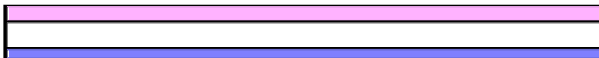
Figure 3: a transdermal drug delivery patch without a drug reservoir. From the top the different layers are: the backing, a drug carrying pressure sensitive adhesive and a release liner. The release liner takes care of a constant diffusion rate of the drug through the skin.
